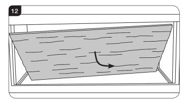
3a.9 Replace the liners in reverse order using the same technique to ensure no damage occurs.
