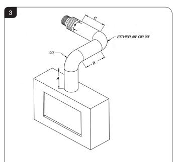
When A = 1.0 to 1.499 metres B + C = 1.0 metres maximum When A = 1.5 metres to 1.999 metres B + C = 2.0 metres maximum When A = 2.0 metres to 3.0 metres B + C = 4.0 metres maximum
