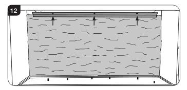
3a.8 Carefully remove the back liner by tilting the top forward and lifting slightly to clear the burner tray. Twist slightly to allow it to be removed through the front of the appliance, see Diagram 13.
