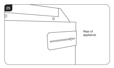
5.13 Remove the screw and rotate the fixing brackets on the appliance so they can be fastened to the wall. Secure in the new position with the screw, see Diagram 26.
