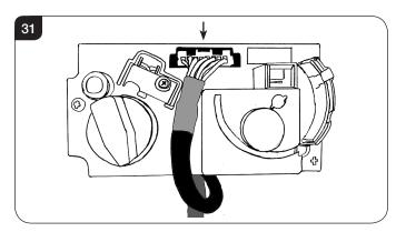
When replacing the 8 way cable ensure that the excess cable is placed between the Control Box and the metal shield, see Diagram 32. Do no allow the cable to touch the underside of the Main Control Assembly.
