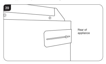
5.44 Remove the screw and rotate the fixing brackets on the appliance so they can be fastened to the wall. Secure in the new position with the screw, see Diagram 40.
