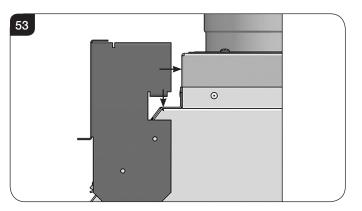
6.23 The rear folded return will sit on the top edges of the appliance below the flue exit. When correctly positioned the front lip of the bracket should be in line with the front face of the appliance and the bracket be level with the top of the airduct see Diagram 54.
