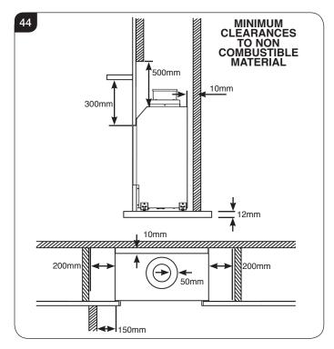
6.3 DO NOT PACK THE VOID AROUND OR ABOVE THE APPLIANCE WITH INSULATION MATERIALS SUCH AS MINERAL WOOL.
