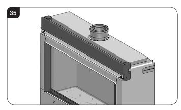
5.37 Line the sides of the tile bracket up with the edges of the Eclipse outer casing, see Diagram 36.
