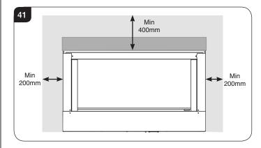
5.49 Non-combustible board above the appliance will rest on the front lip of the tile support bracket leaving a gap of 50mm between the appliance flange and the start of the studwork enclosure.
