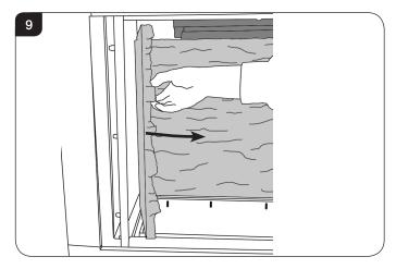
3a.4 Use a lifting motion to pull free of the rear liner whilst simultaneously angling the bottom of the panel upwards to gently withdraw it through the front of the appliance, see Diagram 10.
