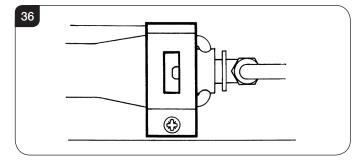
This appliance has 2 venturi. Ensure the correct aeration plates are fitted.
