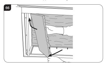
10a.6 Hold the liner by the edge and push flat against the side of the appliance. Slide the panel on the support and the brick effect can lock with the back liner, see Diagram 67.
