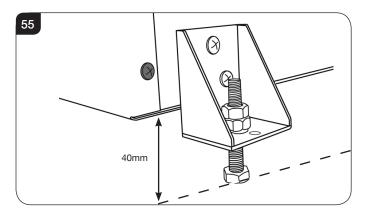
6.28 Fixing brackets are attached to each side of the rear of the appliance by a screw, see Diagram 56.
