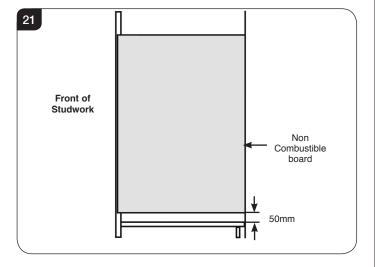
5.9 The 50mm gap allows the air to circulate into the enclosure and cool the appliance, see Diagram 22.
