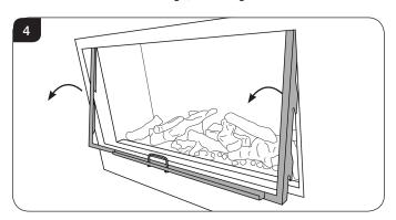
2.7 To replace the glass frame, position so the hooks on the back of the frame fit over the side pins, see Diagram 5.
