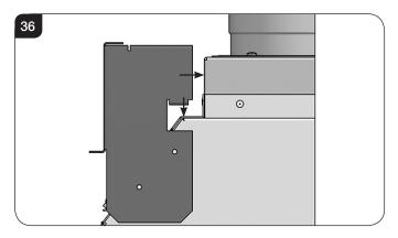
5.38 The rear folded return will sit on the top edges of the appliance below the flue exit. When correctly positioned the front lip of the bracket should be in line with the front face of the appliance and the bracket be level with the top of the airduct see Diagram 37.
