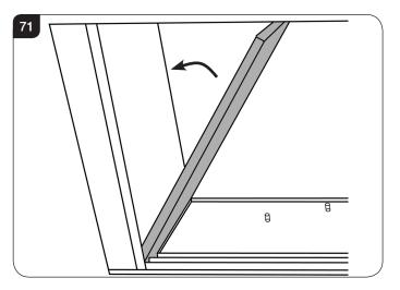
10b.4 Secure the side panels with the brackets at the top. These will need to be loosened and rotated before panels are fitted.
