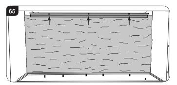
10a.4 The side liner panels are labelled left and right. It is essential to ensure the correct liner is used for each side to allow the brick effect to interlock.
