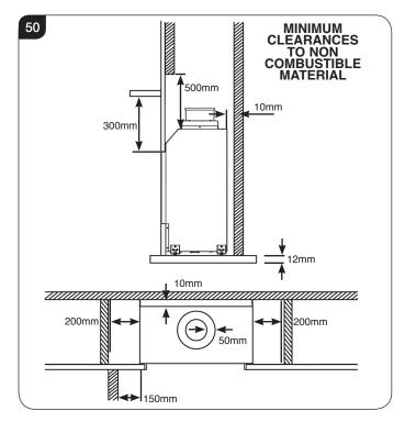
6.19 DO NOT PACK THE VOID AROUND OR ABOVE THE APPLIANCE WITH INSULATION MATERIALS SUCH AS MINERAL WOOL.
