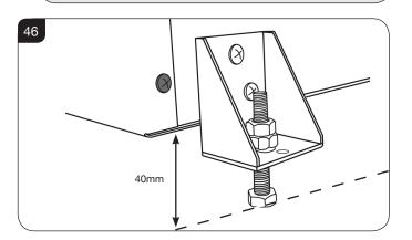
6.6 Fixing brackets are attached to each side of the rear of the appliance by a screw, see Diagram 47.
