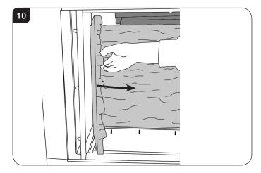
3a.4 Use a lifting motion to pull free of the rear liner whilst simultaneously angling the bottom of the panel upwards to gently withdraw it through the front of the appliance, see Diagram 11.
