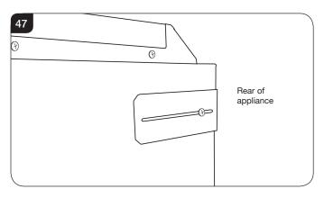
6.7 Remove the screw and rotate the fixing brackets on the appliance so they can be fastened to the wall. Secure in the new position with the screw, see Diagram 48.
