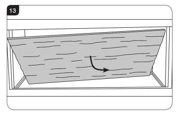
Replace the liners in reverse order using the same technique to ensure no damage occurs.
