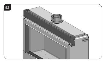
6.22 Line the sides of the tile bracket up with the edges of the Eclipse outer casing, see Diagram 53.
