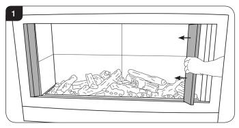
2.3 Lift out the bottom slotted trim, see Diagram 2.
