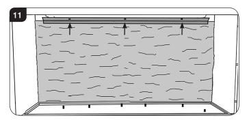
3a.8 Carefully remove the back liner by tilting the top forward and lifting slightly to clear the burner tray. Twist slightly to allow it to be removed through the front of the appliance, see Diagram 12.
