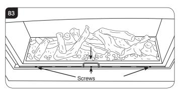
13.3 Replace the screws. As the screws are tightened the glass frame is pulled down against the hooks and forms a seal. Replace ALL of the securing screws ensuring that a screw is present in all fixing slots.
